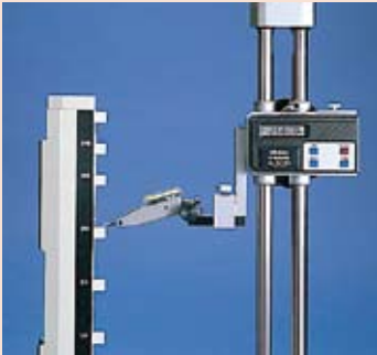
Checking a height gage
