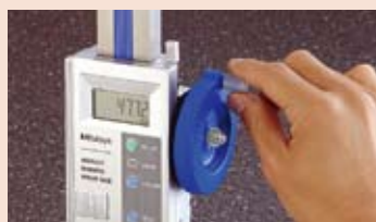
Large smooth slider feed wheel
